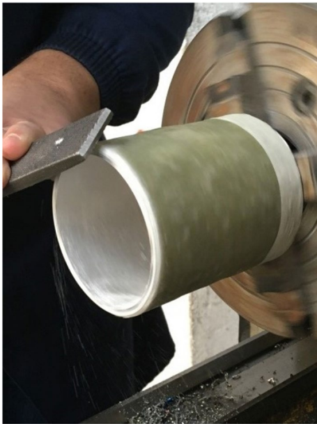
Fig. 6 Chamfering process of the hybrid tube
