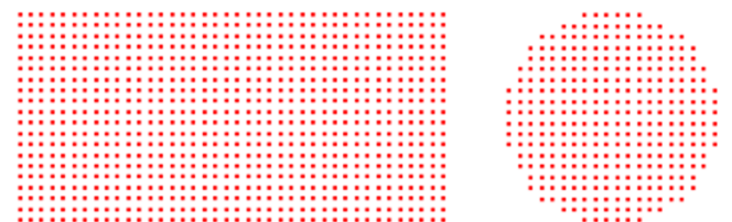
Fig. 10 SPH particle distribution used to model the bird body (side and front views).
