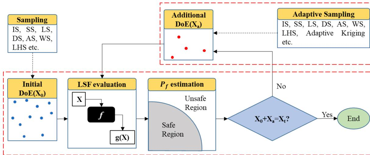
**Fig. 3** General framework for sampling-based methods for estimation of small failure probability.  $X_0$  is the initial sample,  $X_a$  is the adaptive or additional sample and  $X_t$  is the total samples available for LSF evaluation or budget in terms of LSF
