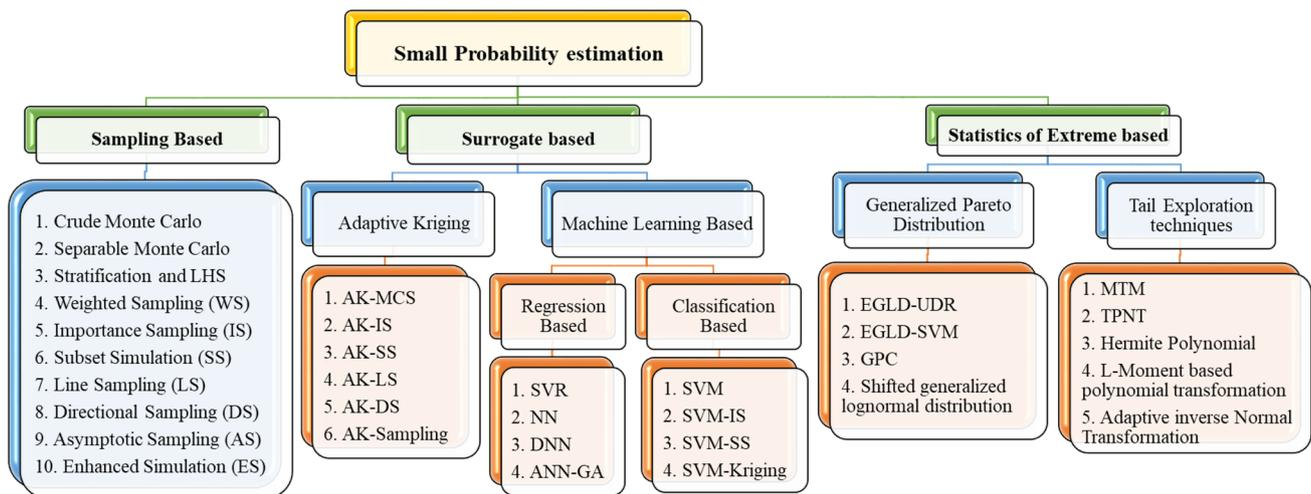
Fig. 2 Brief categorization of the approaches for estimation of small failure probability
