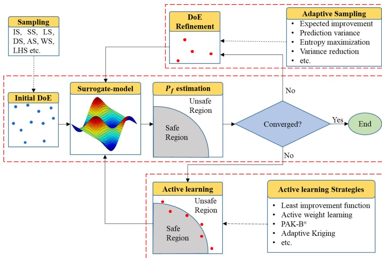
Fig. 4 General framework for surrogate-based techniques for small failure probability estimation
