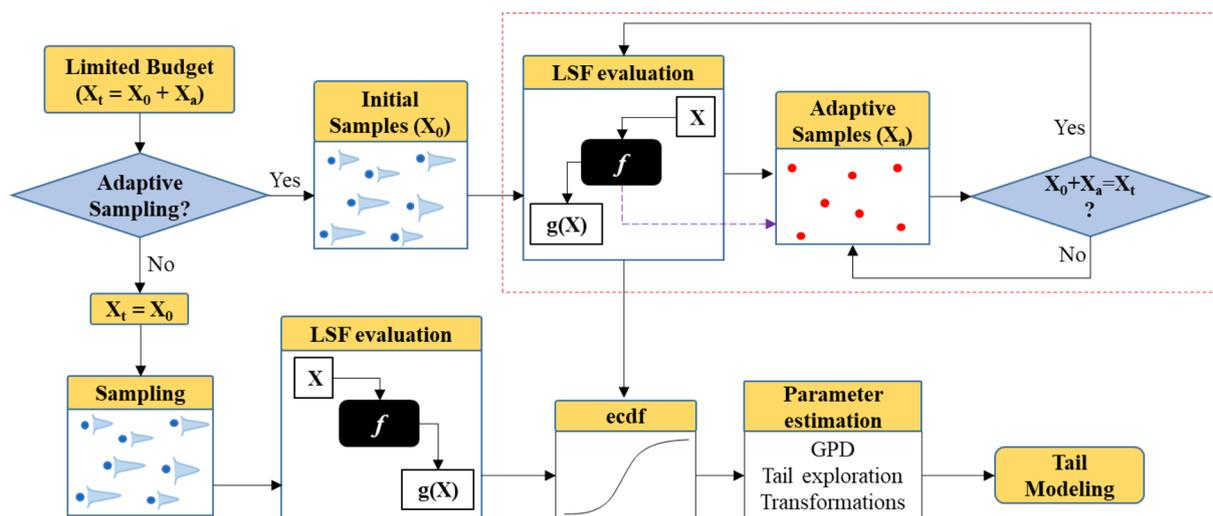
Fig. 8 General framework for statistics of extreme-based methods for estimation of small failure probability.  $X_0$  is initial sample,  $X_a$  is the adaptive or additional sample and  $X_t$  is total samples available for LSF evaluation or budget in terms of LSF
