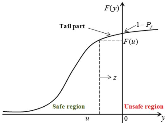
Fig. 7 Concept of GPD for tail modeling
