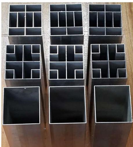
**Fig. 2** Geometric views and manufactured test specimens for different tube configurations **a** single-cell (T0) **b** multi-cell (T4E) **c** multi-cell (T8E)
