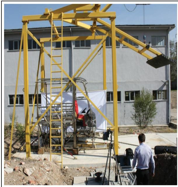
**Figure 10.** Crash test including pendulum and bus structure.
