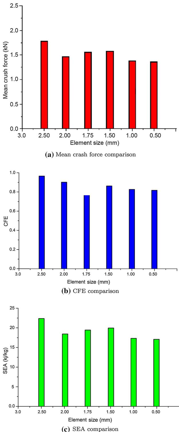
**Fig. 7** Mesh convergence study for the FE model of the honeycomb structure
