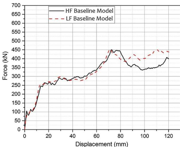
**Fig. 16** Comparison of the low-fidelity (LF) and high-fidelity (HF) models based on the force–displacement behavior for the baseline model
