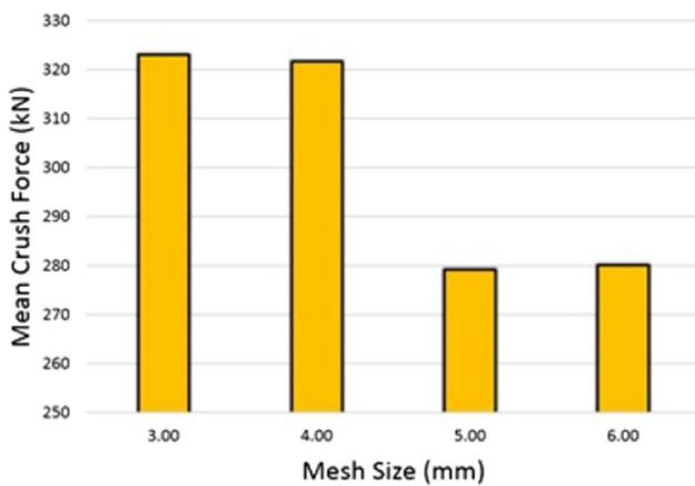
Fig. 12 Mean crush force comparison for different mesh sizes of bumper beam and crashboxes
