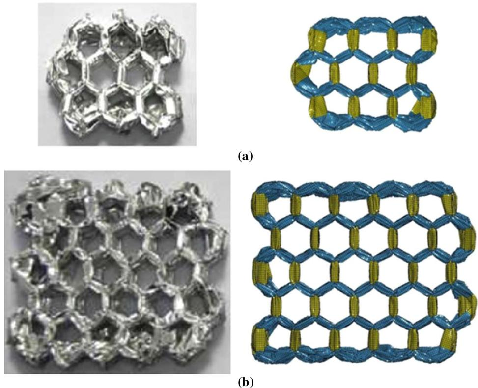
**Fig. 11** Finite element setup
