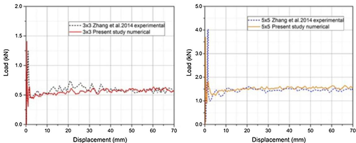
**Fig. 9** 3 × 3 cell configuration (on the left), 5 × 5 cell configuration (on the right). Load–displacement graph comparisons of FE analyses and experimental results of Zhang et al. [55]
