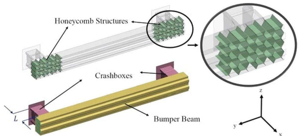
**Fig. 3** Dimensions of the bumper system
