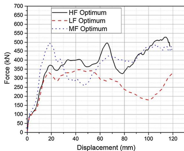
**Fig. 18** Force–displacement responses of the high-fidelity model at optimum points
