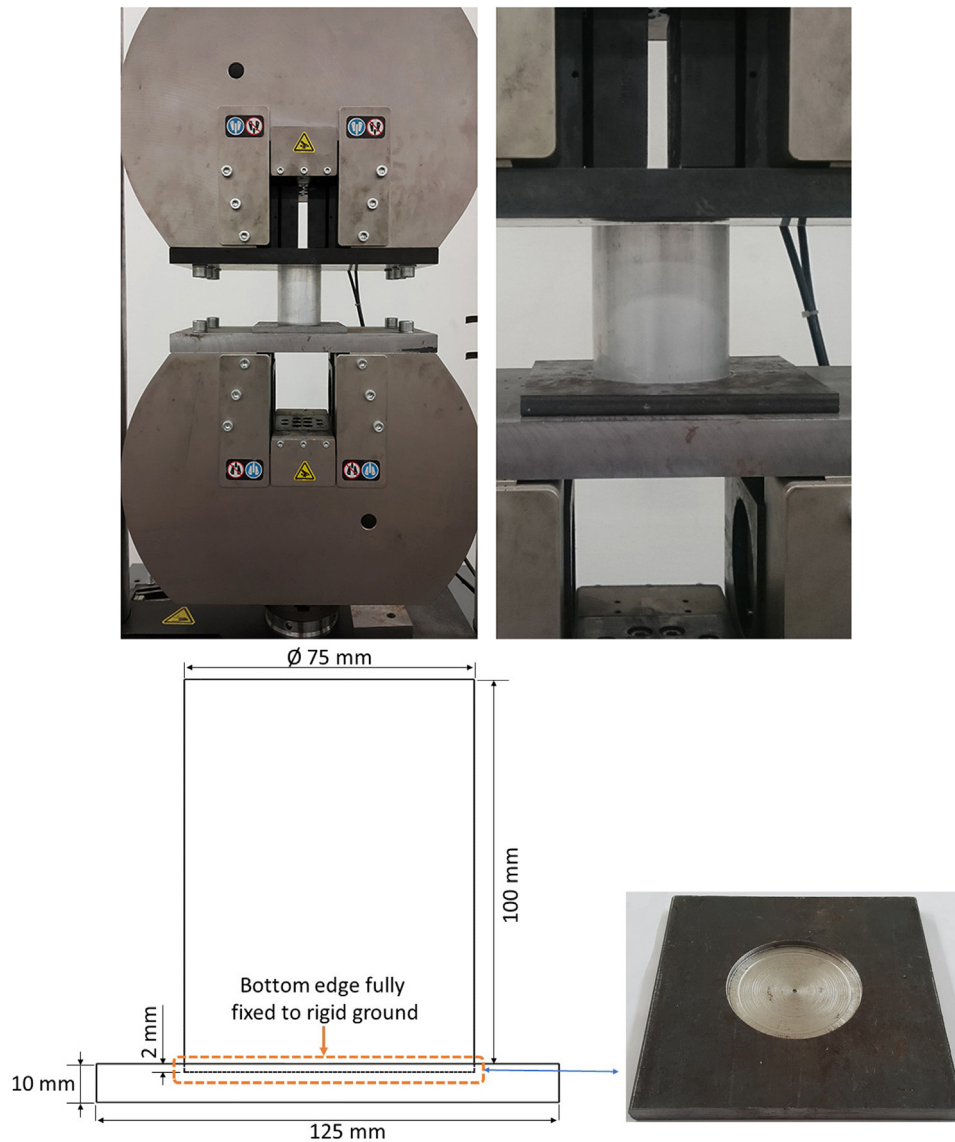
Fig. 12. Quasi-static axial compressive test for empty column (courtesy of Altin et al. [4]).
