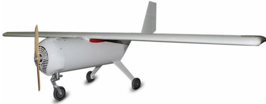
Fig. 2. Unmanned aerial vehicle designed and manufactured in TÜBİTAK 107M103 project.
