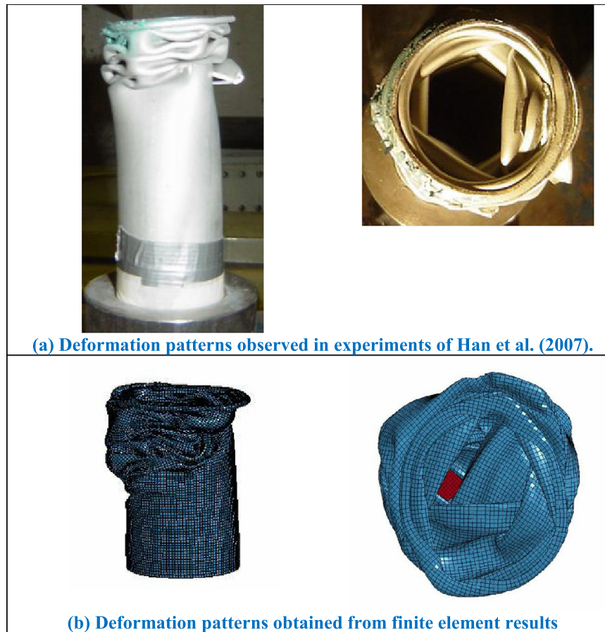
Fig. 7. Comparison of the deformation patterns obtained from the finite element model of the present study to the ones observed in experiments.
