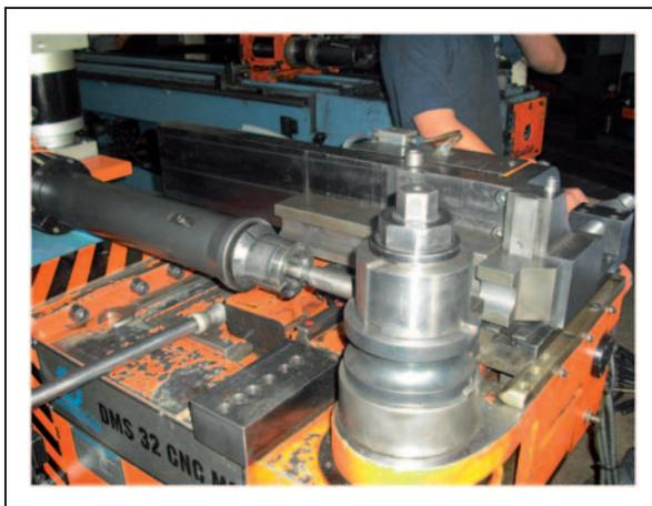
**Figure 10.** CNC rotary-draw tube bender used in the experiments.
