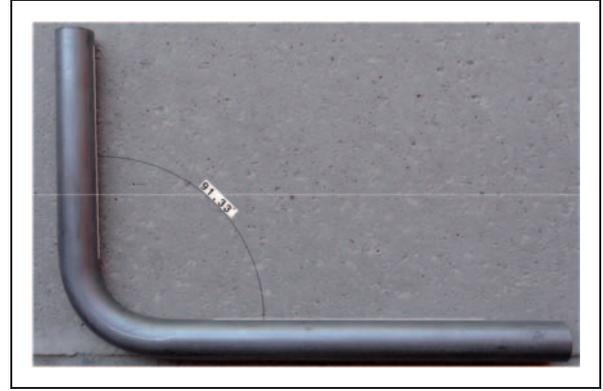
**Figure 12.** Springback measurement from a sample. Material: A573-81 65, bend angle ( $\theta$ ):  $90^\circ$ , bend radius ( $R$ ): 30 mm, tube diameter ( $D$ ): 15 mm, and tube thickness ( $t$ ): 2 mm.
