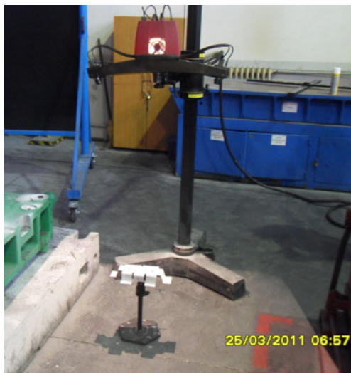
Fig. 4 The experimental springback measurements using ATOS 3D Scanning Software and Systems
