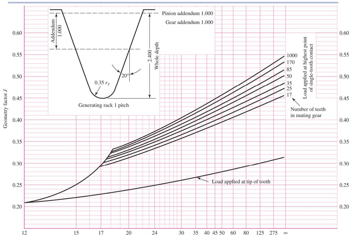
Fig. 14–6 Number of teeth for which geometry factor is desired
