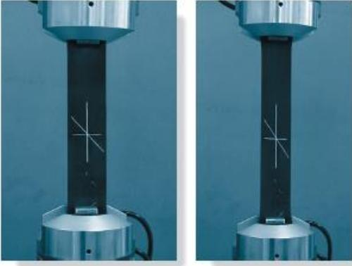
Note the before and after positions of 3 line segments where the material is subjected to tension.
