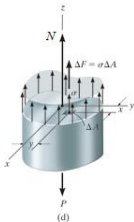
Equations (1) and (2) are automatically satisfied, because  $N$  pass through the centroid, for which  $\int x dA = 0$  and  $\int y dA = 0$ .
