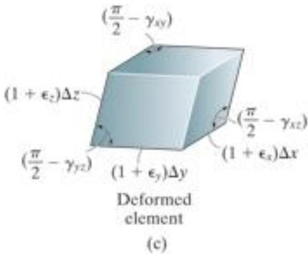
Shear strain components → **shape change**
