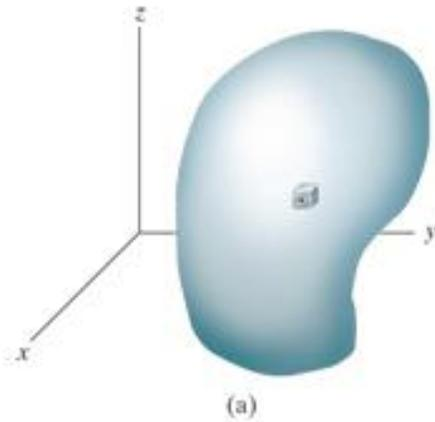
Assume that a deformed body is subdivided into small rectangular elements, and we concentrate on such an element
