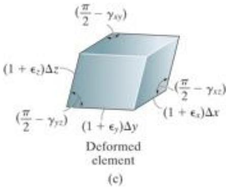
Shear strain components → **shape change**
