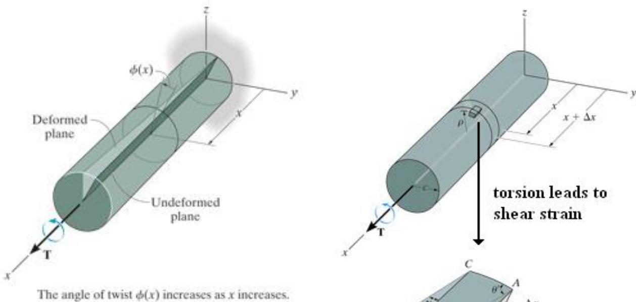
The angle of twist  $\phi(x)$  increases as  $x$  increases.
