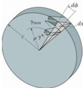
Shear strain linearly changes with
