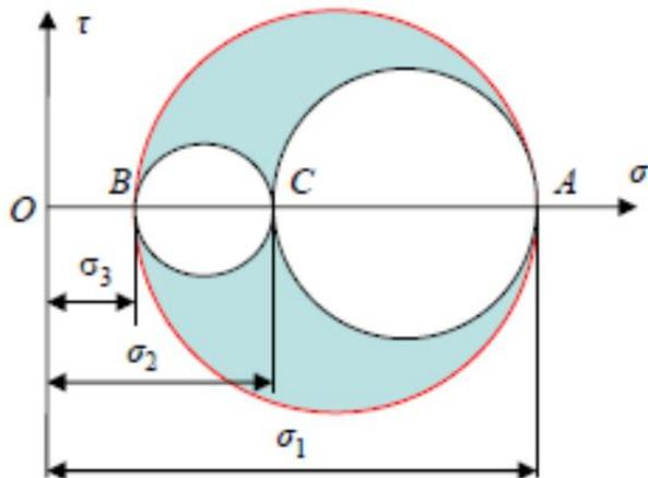
The absolute maximum shear stress and the corresponding average stress are calculated from
