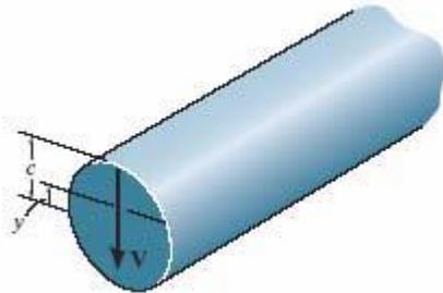
**Example 3:** Calculate the shear stress distribution over the section shown
