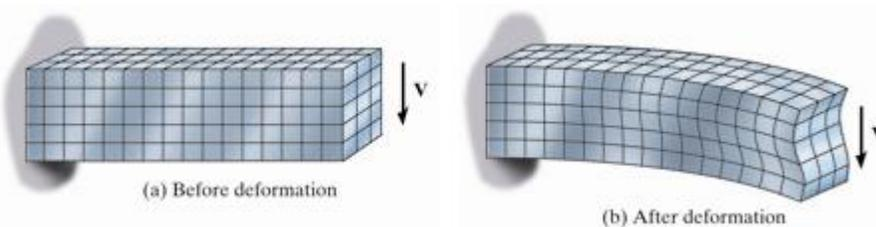
For axial loading, the strains are constant. Similarly, for bending and torsion, the strains are linear. Thus, we were able to start from strain distributions to compute stresses.
